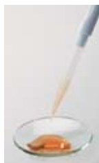
Air displacement pipette: viscous liquid adheres to the inside wall of the tip
