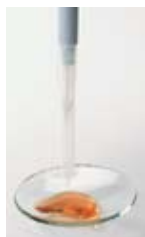
Positive displacement pipette: no viscous liquid remains in the capillary piston
