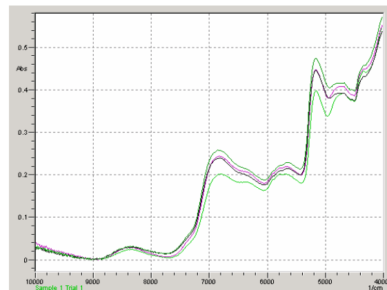
Figure 2: The FT-NIR spectra of the calibration set illustrate the general trend between absorbance and the number of sprays.
